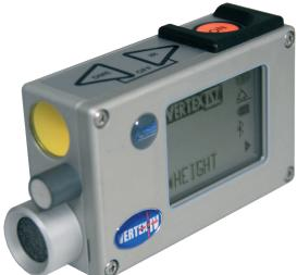
To define a reference point in a secure and reliable way, the Vertex IV works with the transponder T3. The Vertex IV communicates with the transponder. This communication eliminates in an efficient way any mix-
