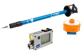
at optional heights, where visibility is the best in for example thick vegetation. The reference point height (T.HEIGHT in Vertex instrument setup) is set in a special menu in the Vertex instrument and automatically added to the measured height.
