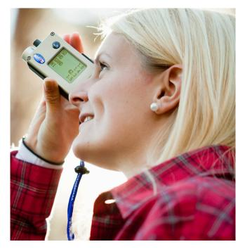
Ultrasound is a well proven technique that works for measurement work in the forest. The Vertex IV uses ultrasound to measure distances. Unlike measuring tapes and laser instruments, ultrasound works when the reference point is obscured and covered by shrubs, branches and leaves.
