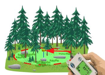
The ultrasound signals can be used also when the target is covered by shrubs and undergrowth. Tree heights are calculated as a compensated value with the variables obtained when measuring angle and distance. Use the Vertex IV with the transponder T3 pinned to the tree or mounted on the custom plot staff and adapter.
